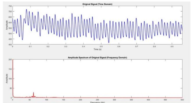
**FIGURE 20.** analysis PPG signal uses FFT
