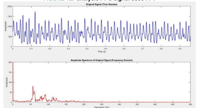
FIGURE 13. analysis PPG signal uses FFT
