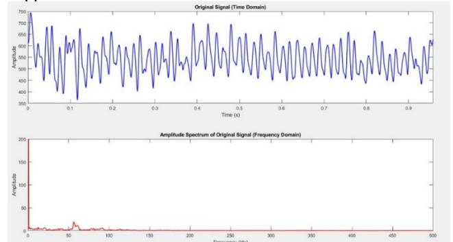
FIGURE 12. analysis PPG signal uses FFT
