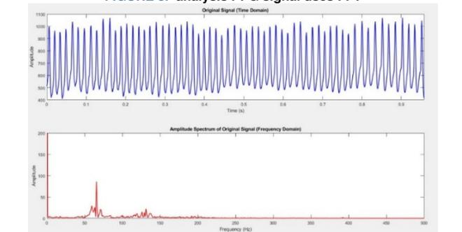
FIGURE 9. analysis PPG signal uses FFT
