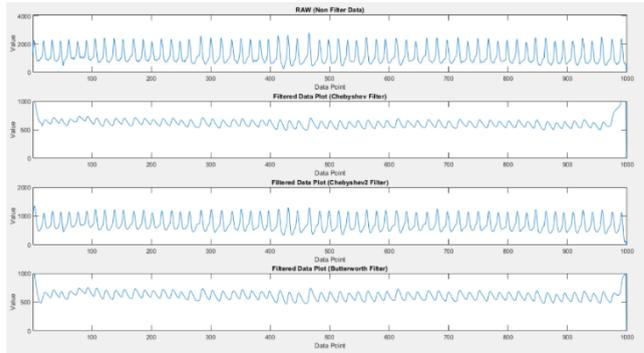
**FIGURE 16.** Plotting of the PPG signal during filter testing when making finger waving movements
