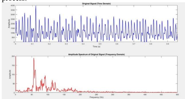
FIGURE 9. analysis PPG signal uses FFT
