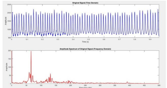
FIGURE 7. analysis PPG signal uses FFT
