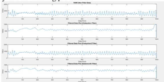
FIGURE 11. Plotting of the PPG signal during filter testing when performing finger movements 0 – 90 degrees
