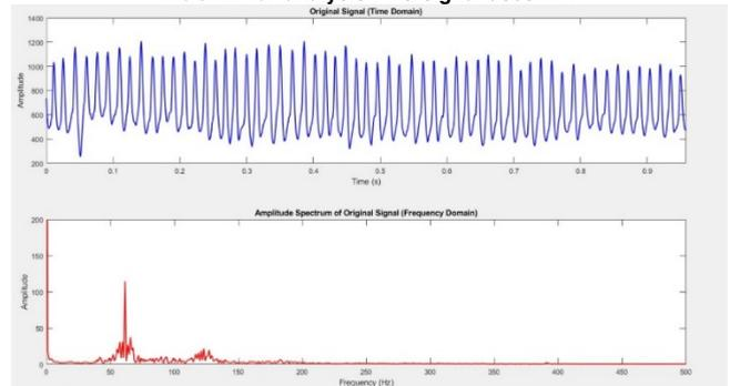
**FIGURE 19.** analysis PPG signal uses FFT
