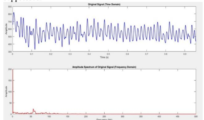
FIGURE 14. analysis PPG signal uses FFT
