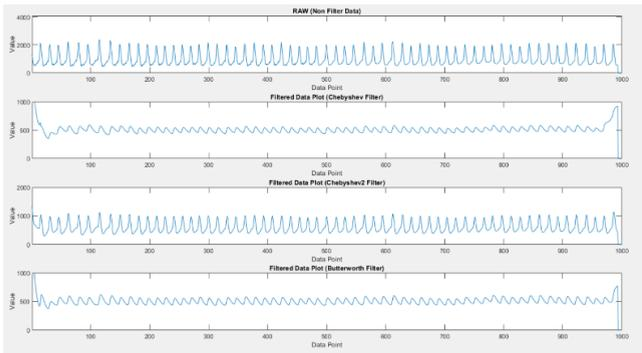
FIGURE 6. Plotting of the PPG signal during filter testing when not moving
