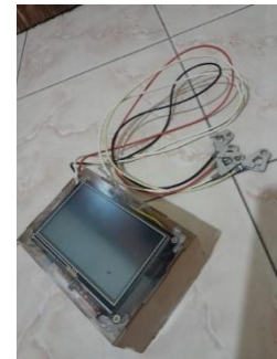
Figure 3. ECG Monitoring Module Equipped with 4 Electrodes
