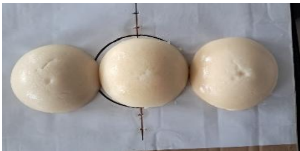
Figure 7. Condition of the fabricated heterogeneous breast phantom after 10 weeks of storage.
