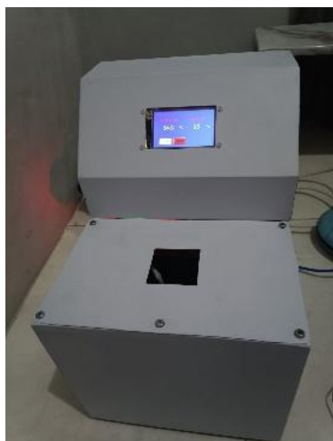
Fig. 2. Thermogun Calibrator with Fuzzy-PID Control
